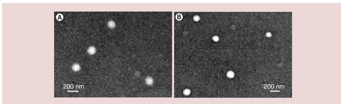
**Figure 1. Morphology of the developed lipid nanoparticles.** Transmission electron microscopy images of (A) nanostructured lipid carriers and (B) mannosylated-nanostructured lipid carriers, at 50,000× magnification. The white bar represents 200 nm.
