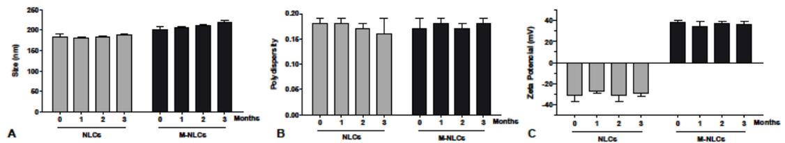
**Supplementary Figure 1. Storage stability of A) hydrodynamic particle size, B) polydispersity index, and C) zeta-potential of NLCs and M-NLCs, during 3 months of storage at 20°C. Data expressed as mean  $\pm$  SD (n=3).**
