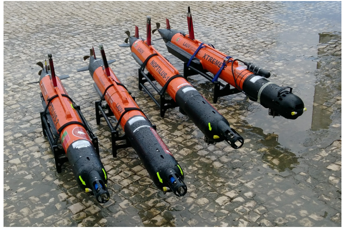
Fig. 1. Bottom-mapping LAUV vehicles. The rightmost AUV (LAUV-Xtreme-2) is equipped with Sidescan sonar, video camera and self-compensating magnetometer.
