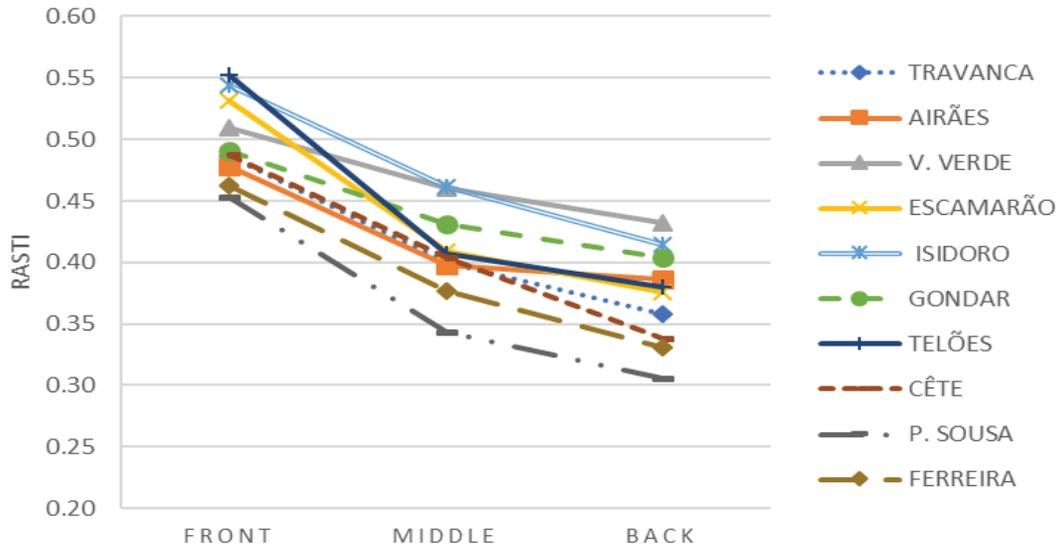
Figure 10 – Mean *RASTI* values measured in each of the three zones (as in figure 8) of each sampled church.
