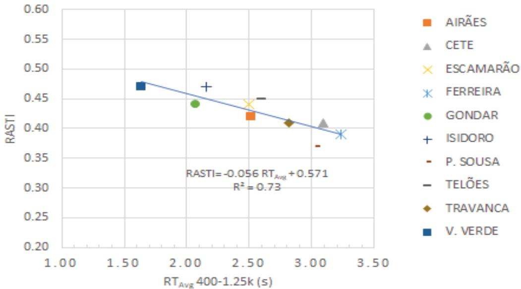
Figure 13 – Relationship between mean  $RASTI_{avg}$  and  $RT_{avg}(400-1.25k\text{ Hz})$  values
