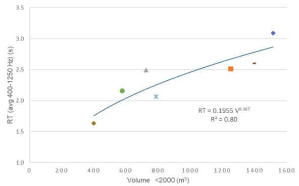
Figure 11 (left) - Relationship between  $RT_{avg}(400-1.25k\text{ Hz})$  and  $Volume$  for each church
