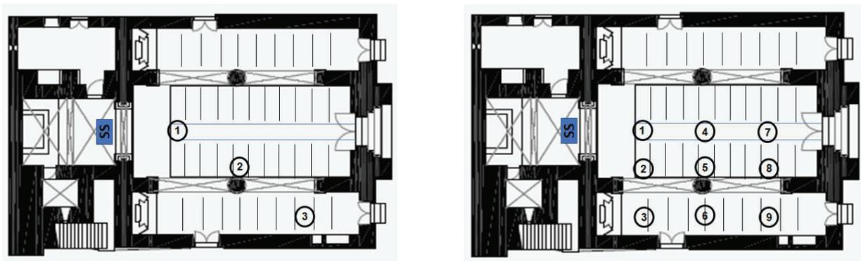
Figure 7 (left) – The three typical *RT* measurement positions in each church, *SS* (sound source)
