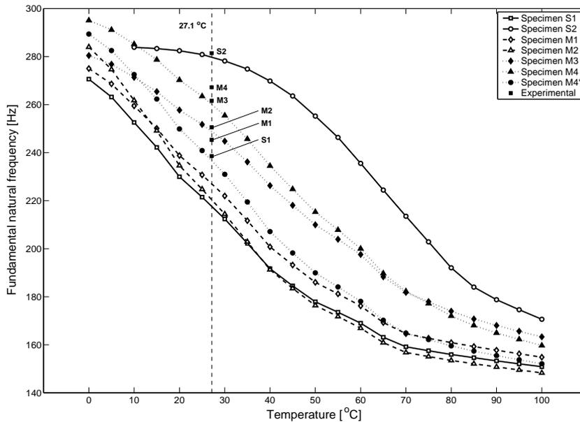
Figure 12. Fundamental natural frequency distribution
