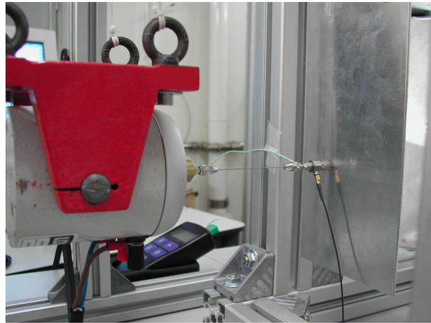
Figure 4. Experimental setup - specimen excitation
