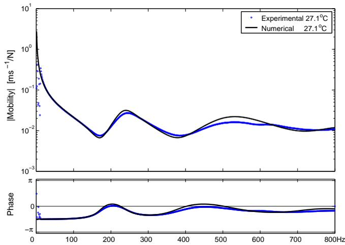
Figure 6. Direct mobility function for specimen S1 (27.11°C)
