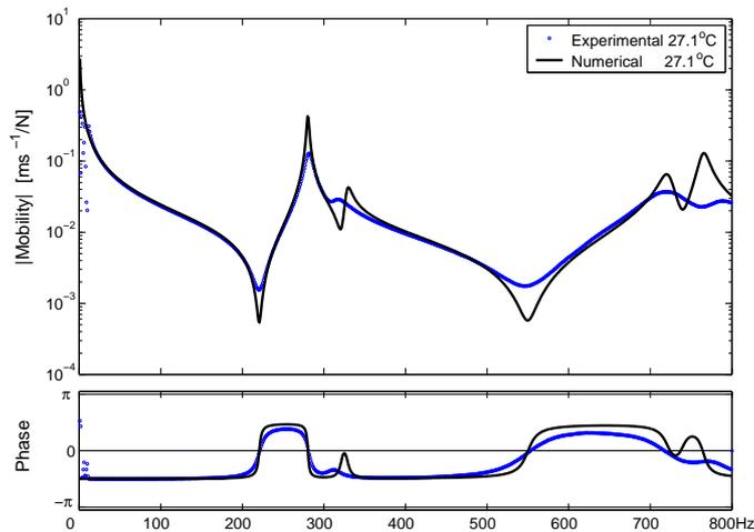
Figure 7. Direct mobility function for specimen S2 (27.11°C)
