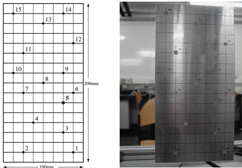
Figure 3. Measuring mesh and specimen boundary conditions
