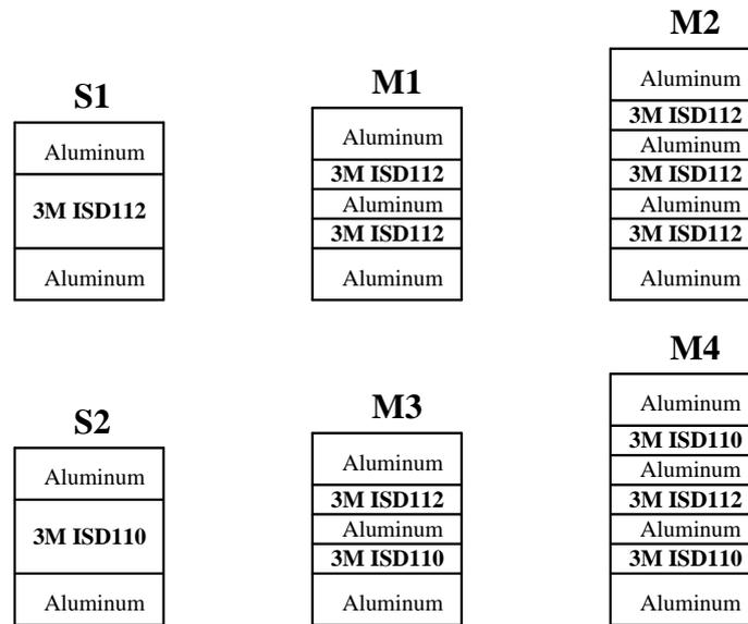
Figure 1. Specimens configuration
