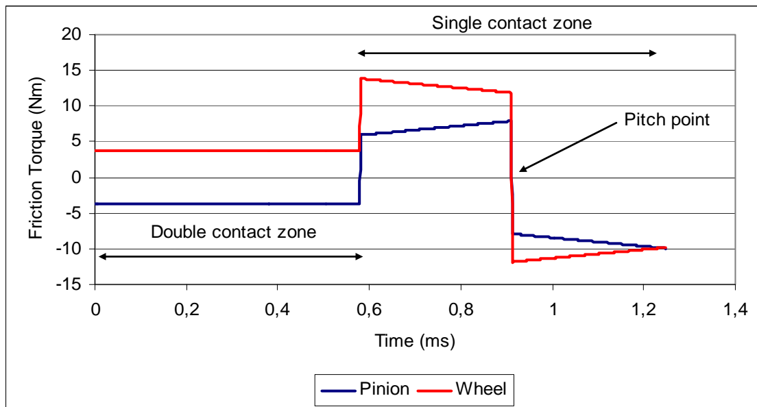
Figure 4. Example of pinion and wheel friction torques along line the meshing line.
