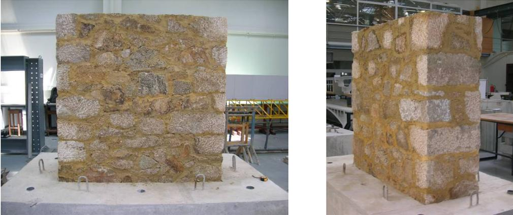
Figure 1: The stone masonry wall specimen.
