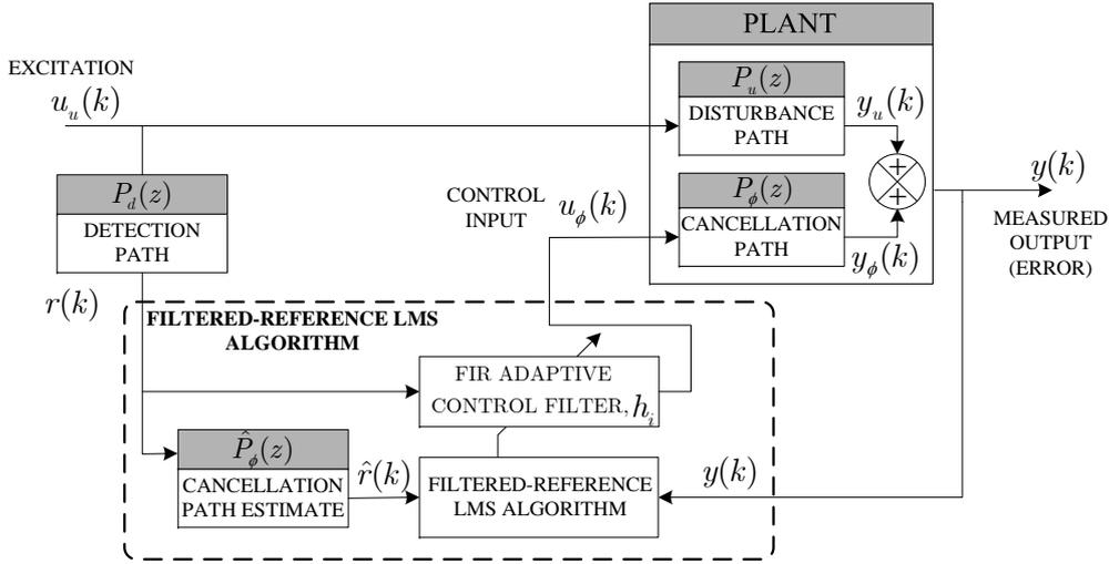
Figure 1: Schematic of the discrete-time (digital) generalized plant for a feedforward SISO controller.
