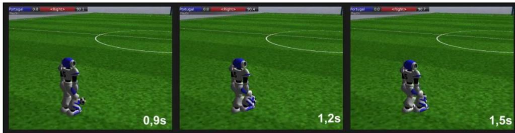
Figure 16. Sequence of the lowering and placing support foot
