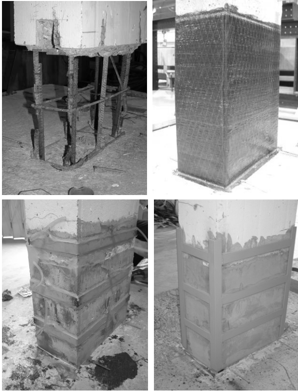
Fig. 13. Lap spliced zone (up-left); retrofitted column with CFRP sheet jacket (up-right); steel plates (down-left); and steel plates connected by equal leg angle steel profiles (down-right).
