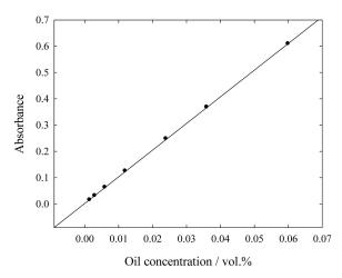
Fig. 6. Calibration curve: absorbance versus oil concentration.
