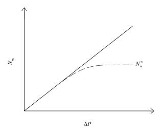
**Fig. 2.** Permeate flux versus pressure difference: continuous line—linear relationship (Equation (1)); dashed line—deviation from Equation (1) caused by the occurrence of concentration polarization phenomenon, where a limiting flux is obtained  $(N_w^{\infty})$ .
