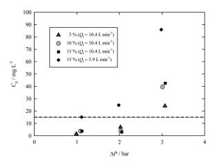
**Fig. 9.** Oil permeate concentration as a function of the pressure difference across the membrane for different feed oil concentration and feed flow rates. The dashed line stands for the Portuguese limit value of oil concentration in wastewaters.
