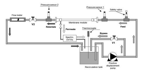
Fig. 3. Schematic representation of the experimental set-up.
