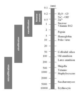
**Fig. 1.** Application of the microfiltration, ultrafiltration, nanofiltration and reverse osmosis processes as a function of the membrane pore size; adapted from [4].
