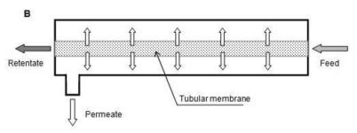
Fig. 4. Streams involved in permeation through a tubular membrane (A) and in a membrane module without sweep stream (B).
