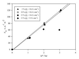
**Fig. 8.** Permeate flux as a function of pressure difference between the feed and permeate sides, for different emulsion concentrations and feed flow rates. Lines show the fitting by linear regression to experimental data (c.f. Equation (2)).
