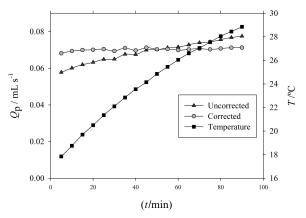
**Fig. 7.** Corrected (due to viscosity variation) and non-corrected permeate flow rate along the time for a 5 vol.% O/W emulsion and a total pressure difference of 1 bar. O/W temperature along the time is also presented. Lines are for eye guidance.
