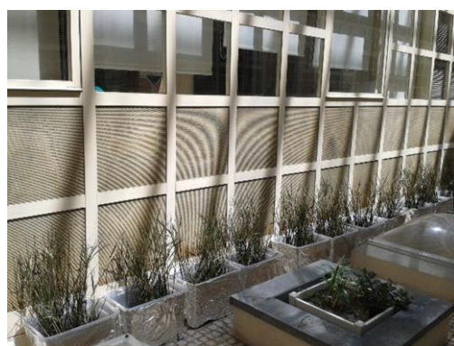
Figure 10: Constructed wetland – microcosm's setup.
