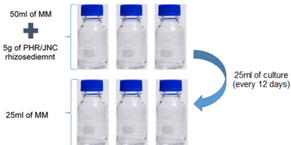
Figure 22: Inoculation and culture setup and maintenance.
