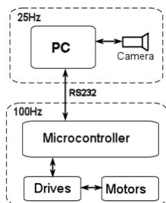
Figure 3: Robot's control and communication structure.
