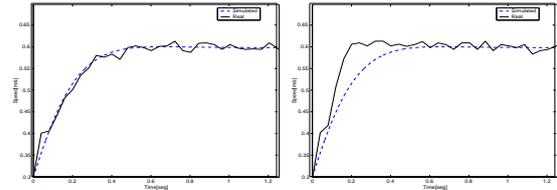
(a) Close-loop system with- (b) Close-loop system with out the *Feedforward* gain  $f$ . the *Feedforward* gain  $f$ .
