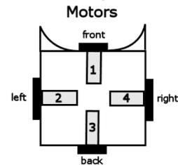
Figure 1: Mobile robot - motors.
