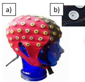
Figure 2. 3: a) EEG head cap with electrodes "already-assembled"; b) Gel-based electrode. Adapted from [129].
