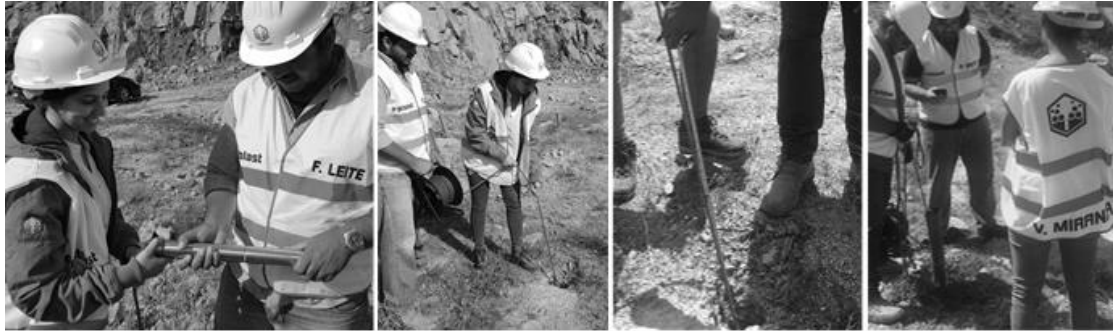
Figure 1: Field Procedure: a) probe assembling; b) probe deployment; c) offset measurement; d) measurement time record
