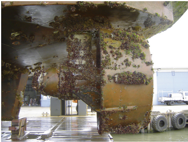
Fig. 1. Vessel hull fouling. Marine biofouling describes the community of organisms that settle and grow on the external surfaces of submerged structures. Within hours of a structure's submergence, a slime layer develops. This layer promotes the settlement and attachment of macro-organisms, including larvae of invertebrates such as ascidians, serpulids and barnacles. Photo: J. Lewis.
