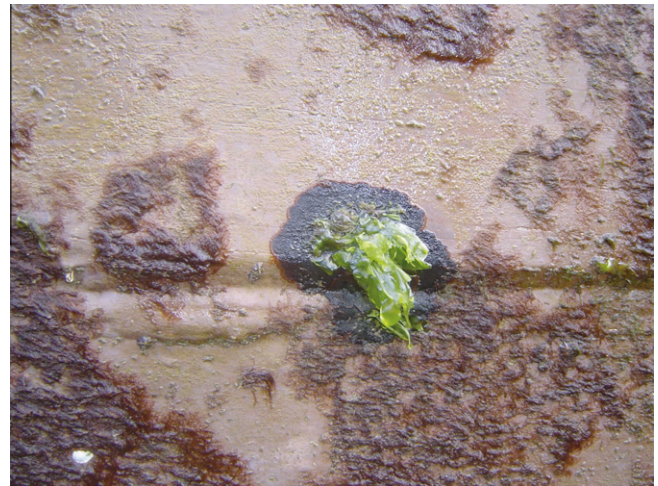
Fig. 3. Positive interactions between fouling species. The non-indigenous bryozoan Watersipora subtorquata is shown growing directly onto a vessel hull coated with copper AF paint and facilitating algal recruitment. Photo: J. Lewis.
