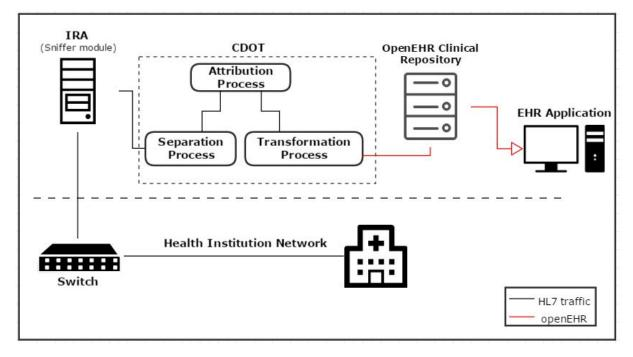
Figure 3.3: Design of the System Architecture of the CDOT and surrounding infrastructure.
