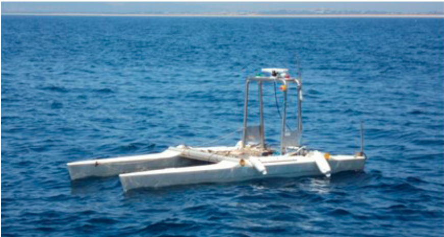
Figure 3: Swordfish Autonomous Surface Vessel developed by LSTS
