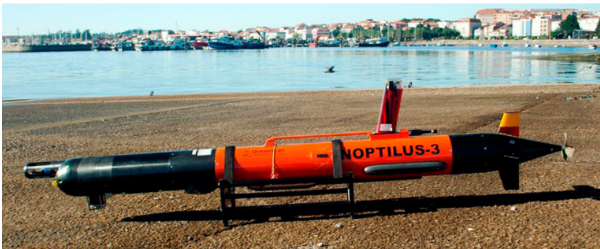
Figure 1: Light Autonomous Underwater Vehicle developed by LSTS
