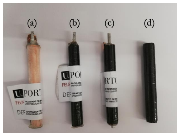
Figure 4. Showcase of the type of coaxial cells and parts investigated; (a) structural battery with thin glass fiber shell such as schematized in Figure 2a; (b) and (c) two coaxial cells that were analysed in this study; (d) CFRP shell.
