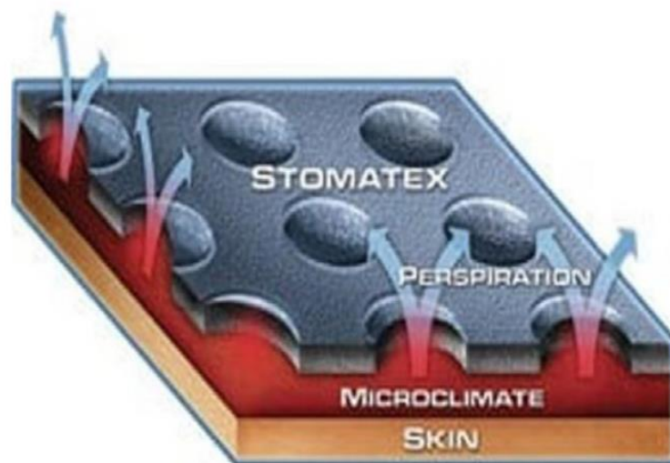
Figure 38: Structure of Stomatex (Maity, Chauhan, & Pandit, 2022)
