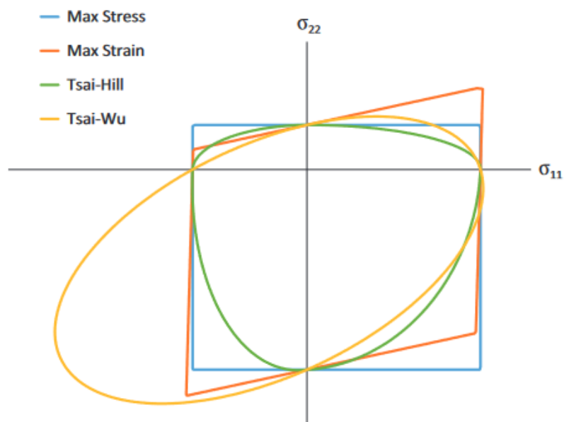
Figure 9: Failure envelopes of the four failure criteria presented (Aboudi, Arnold, & Bednarczyk, 2021)
