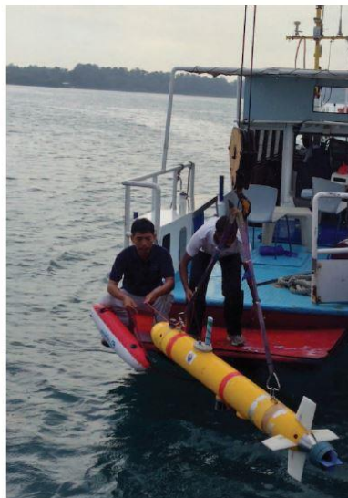
Figure 2.8: The STARFISH AUV being deployed as a mobile network node during the MISSION 2013 experiment [6]
