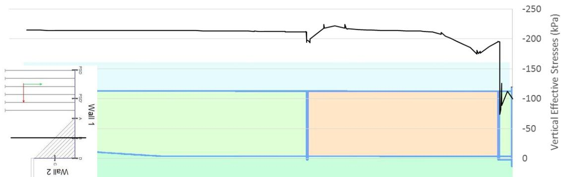
Figure 5.32 - Effective vertical stresses at depth -11m, in a cross section at x=19
