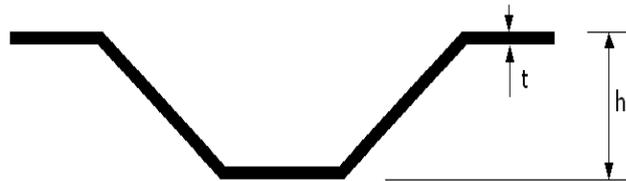
Figure 4.19 - Horizontal cross section of idealized sheet pile
