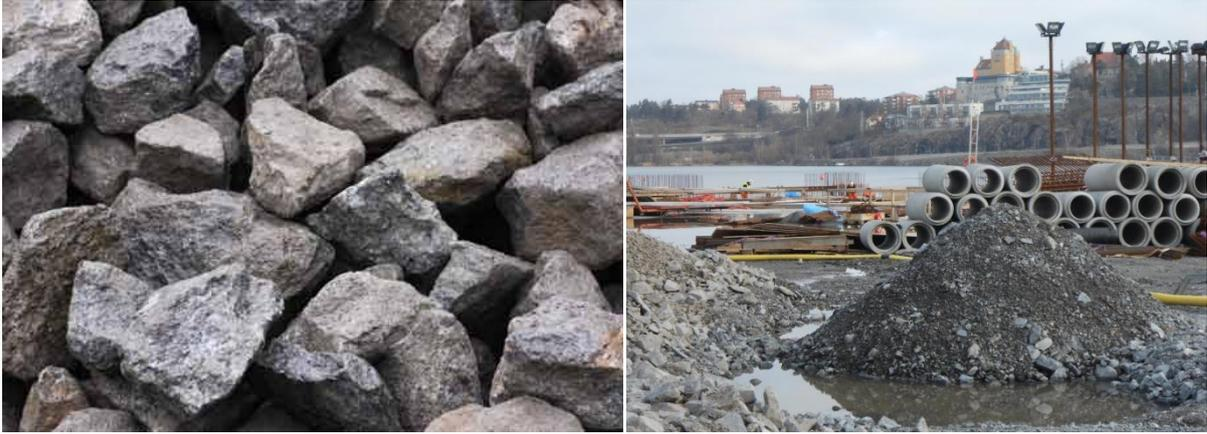
Figure 2.16 - Samples of the *Sprängsten* material used as backfill
