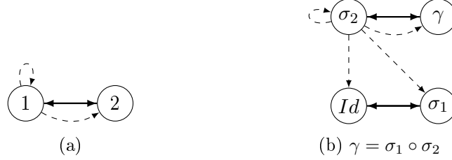
Figure 2.4: (a) Homogeneous network with asymmetric inputs represented by \sigma_1 = [2 \ 1] and \sigma_2 = [1 \ 1] ; (b) Fundamental network of the network (a).
