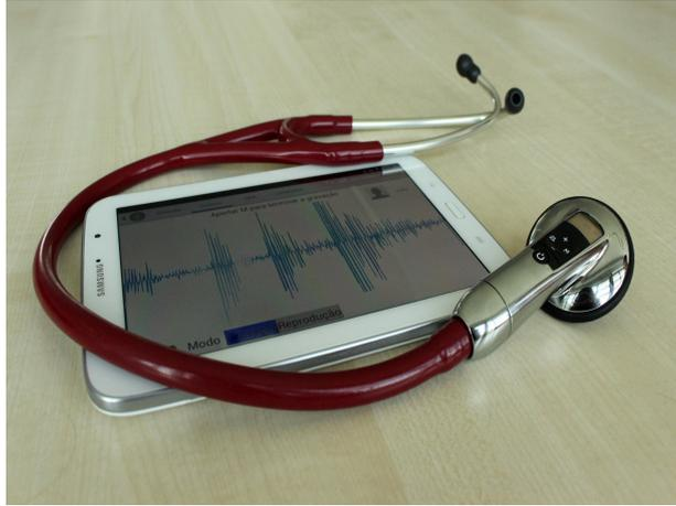
Figure 4.8: Prototype of the DigiScope Collector system, composed by a tablet and an electronic stethoscope Littmann 3200.
