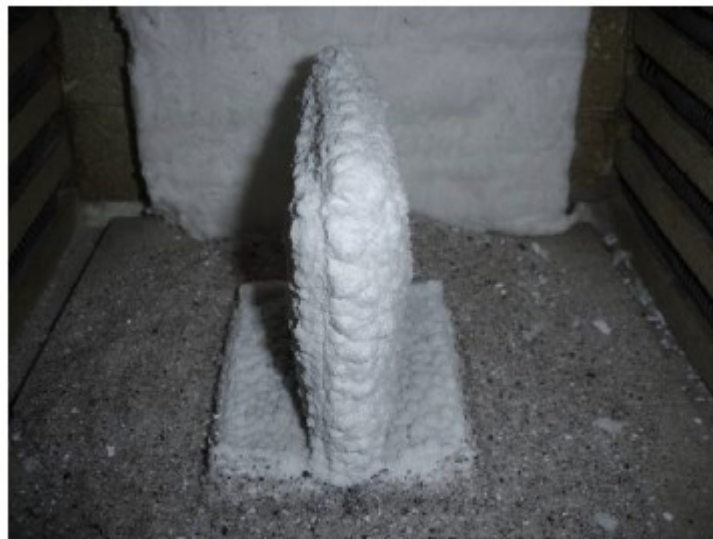
Fig. 2: Example of T steel structure inside the furnace after a thermal insulation test. Notice the white intumescent foam that remained on the structure
