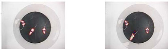
Figure 7: Tracking mice in a lab environment over 414 image frames: quick movement with severe direction changes can be correctly tracked by the proposed tracking framework.
