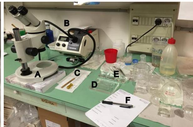
Fig. 12 - Material used to observe and count the zooplankton samples. A - Stereomicroscope type Wild M3 Heerbrugg; B - Stereomicroscope lighting type Olympus KL 1500LCD; C - Dropper pipet and needle; D – Bogorov counting chamber for zooplankton (36mL); E – Glass dishes; F – Protocol.
