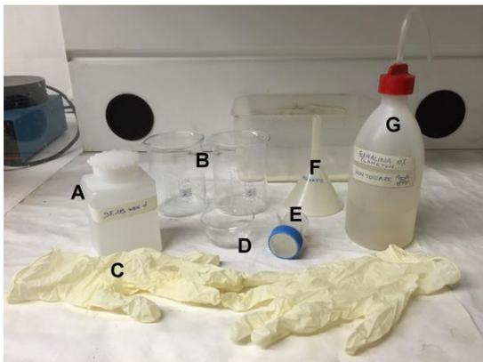
Fig. 11 - Material used to prepare the zooplankton samples. A – Sample bottle (250mL); B –Beaker (250 mL); C – Sterile gloves; D – Evaporating dish; E – 100µm sieve; F – Plastic funnel; G – Bottle with 8% neutralized formalin solution with borax.
