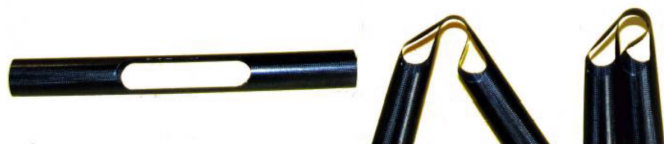
Figure 1: Example of an elastic-hinge, a self-deployable structure in a deployed, partially contracted and fully contracted configuration (figure cited from [7]).
