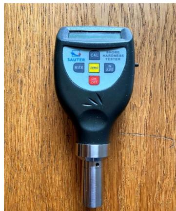
FIGURA 32 - DURÓMETRO
