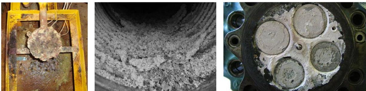
**Figure 2 Acid corrosion, sulphur and silica deposits in engines after exposure to non-purified biogas (Arnold, 2009; BGS, 2018; EPA, 2002).**
