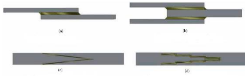
Figure 5 - Adhesive bonded joints configurations: (a) Single lap joint, (b) Double lap joint, (c) Double scarf joint, (d) double stepped-lap joint (adapted from [7]).
