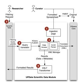
Figure 4: The UPData module architecture
