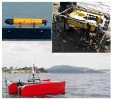
Fig. 7. Isurus (top right), ROV-IES (top left) and Roaz vehicles
