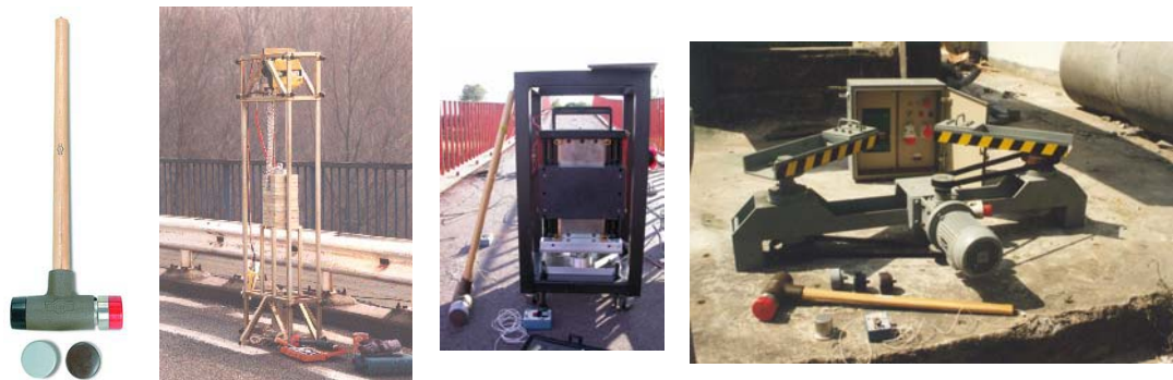
Figure 1. a) Impulse hammer; b) Impulse excitation device for bridges (K.U.Leuven); c) Electrodynamic shaker over three load cells; d) Eccentric mass vibrator.
