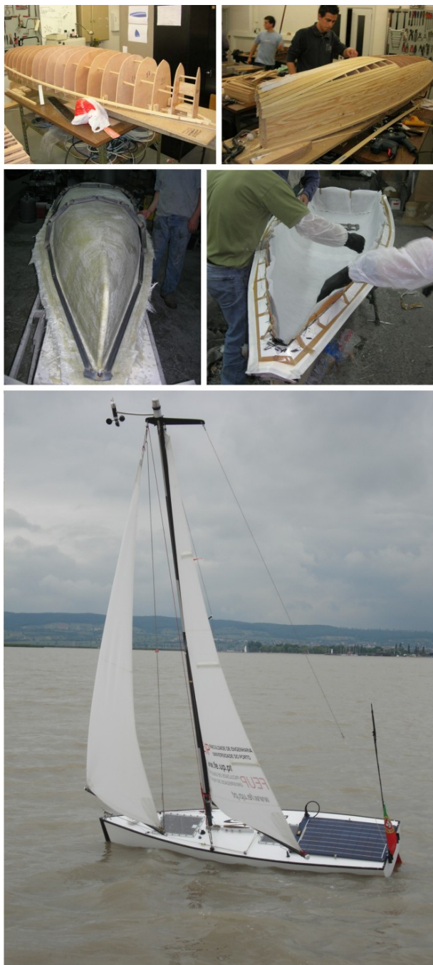
Fig. 1. The construction of FAST: (top-left to bottom) assembly of the frames; strip planking; the mould; building the hull; the final boat.
