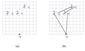
Fig. 2. (a) A mission with three AUVs with their assigned paths and the C3 (b) The route of the UAV meeting the three AUVs and the C3  $\,$
