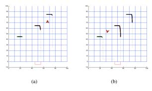
Fig. 5. (a) The new path generated for  $A_2$  at t = 20 sec. (b) After meeting  $A_2$ , the UAV meets  $A_3$  at t = 33 sec and generates a path.
