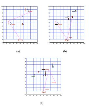
Fig. 6. (a) The predicted route for  $A_2$  and  $A_3$  and the path for  $A_1$  (b) The predicted routes for  $A_1$  and  $A_3$  with the generated new path for  $A_2$ . (3) The predicted route for  $A_1$  and  $A_2$  and the generated path for  $A_3$ .
