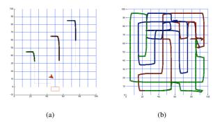
Fig. 7. (a) After meeting  $A_3$  the UAV return to the base station to provide the procured information at t = 44 sec. (b) The paths of the AUVs at the end of the mission.
