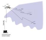
Fig. 1. Scenario of a mission where the command and control center communicates to the AUVs through UAV.
