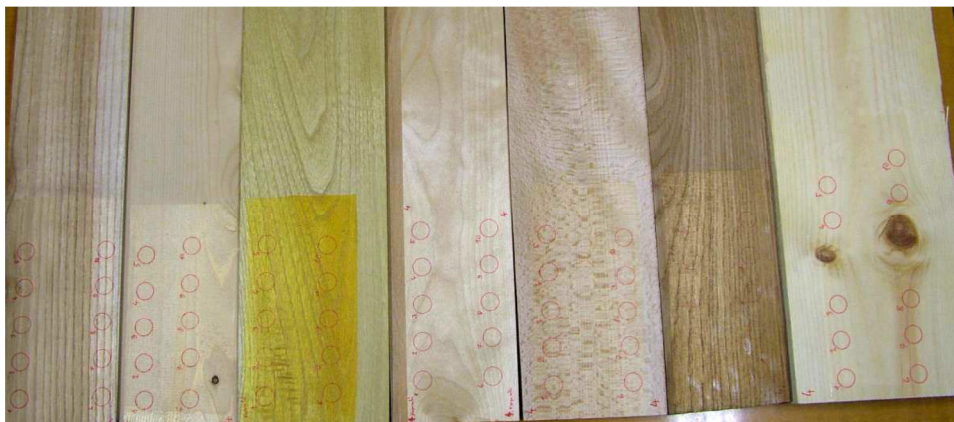
Fig. 1: Discolouration of the wood surfaces after curing the glues and 7 different wood species
