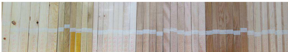
Fig. 3: Change of colour after 1 year storage at indoor conditions for different wood species – with indoor sunlight irradiation
