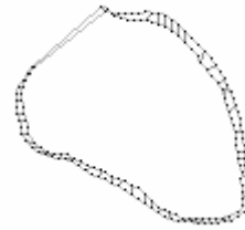
Figure 1: Matching found between two contours “heart5” and “heart6”, using a local search for the correspondences. The contours are defined by 81 and 83 points, respectively.
