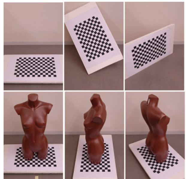
Figure 6. Three images of the sequence used for the intrinsic parameters calibration (above) and three images of the sequence used for the extrinsic calibration parameters (below) for the torso case.
