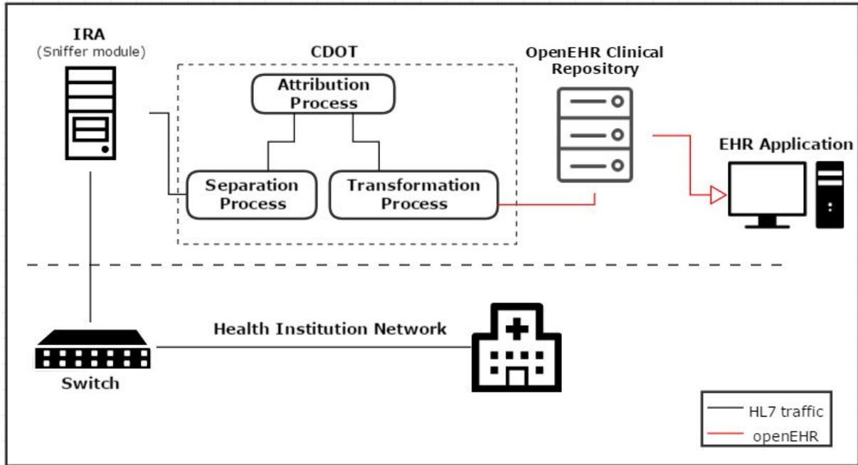
Figure 3.3: Design of the System Architecture of the CDOT and surrounding infrastructure.
