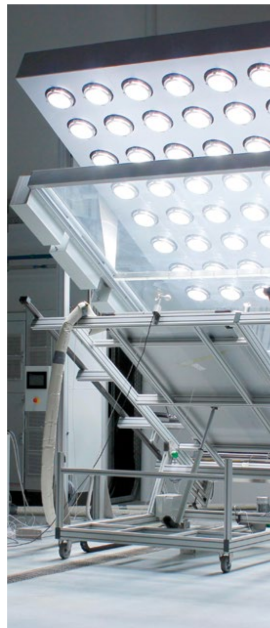
Sistema de teste de painéis solares e revestimentos fotovoltaicos. Cortesia CTCV / Testing system of solar panels and photovoltaic coatings. Courtesy CTCV
