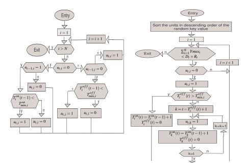
Fig. 3: Minimum up down time repair machanism.
