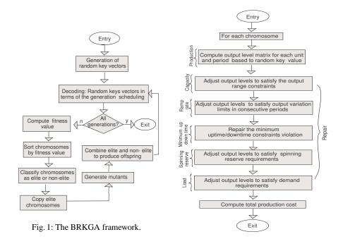
Fig. 2: Flow chart of the decoder.
