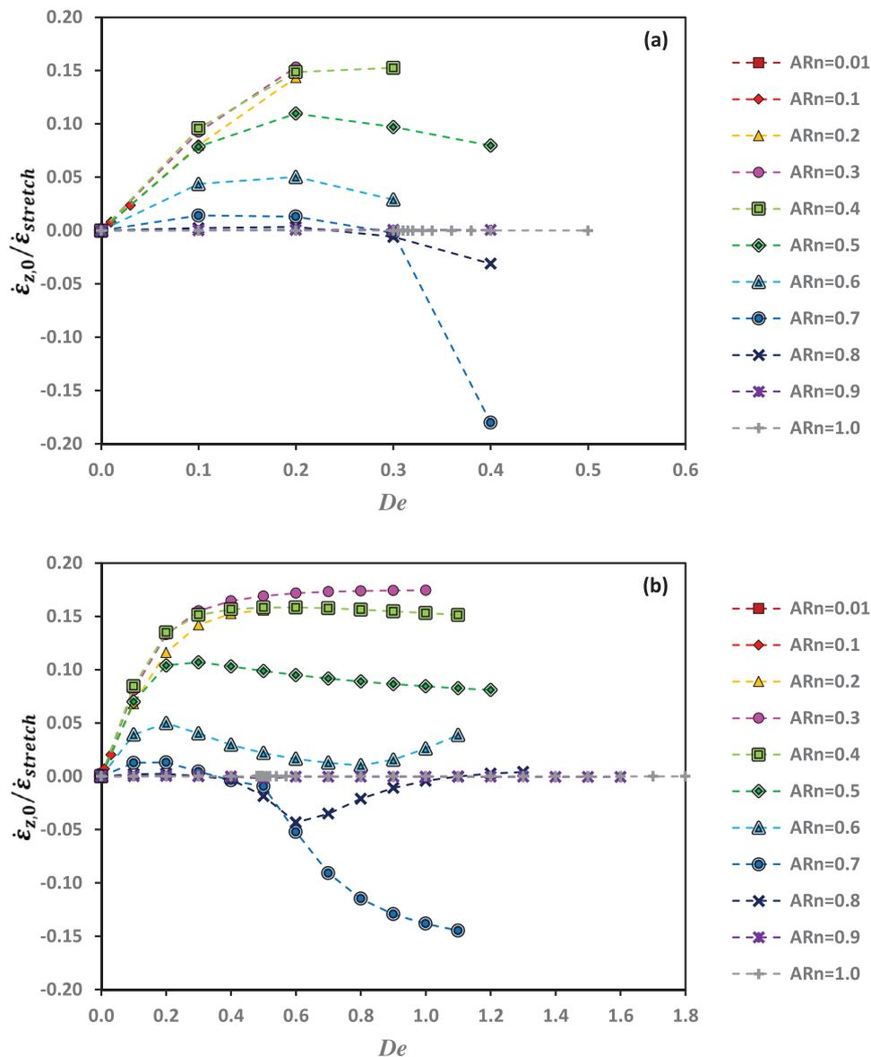
Fig. 7. Strain-rate along the  $z$ -direction at the central stagnation point, normalized by the stretch on the central  $XY$  plane, for the steady state flow of (a) the UCM fluid and (b) the sPTT fluid, with  $\varepsilon = 0.02$  and  $\beta = 1/9$ . Positive values indicate local stretching and negative values represent local compression.
