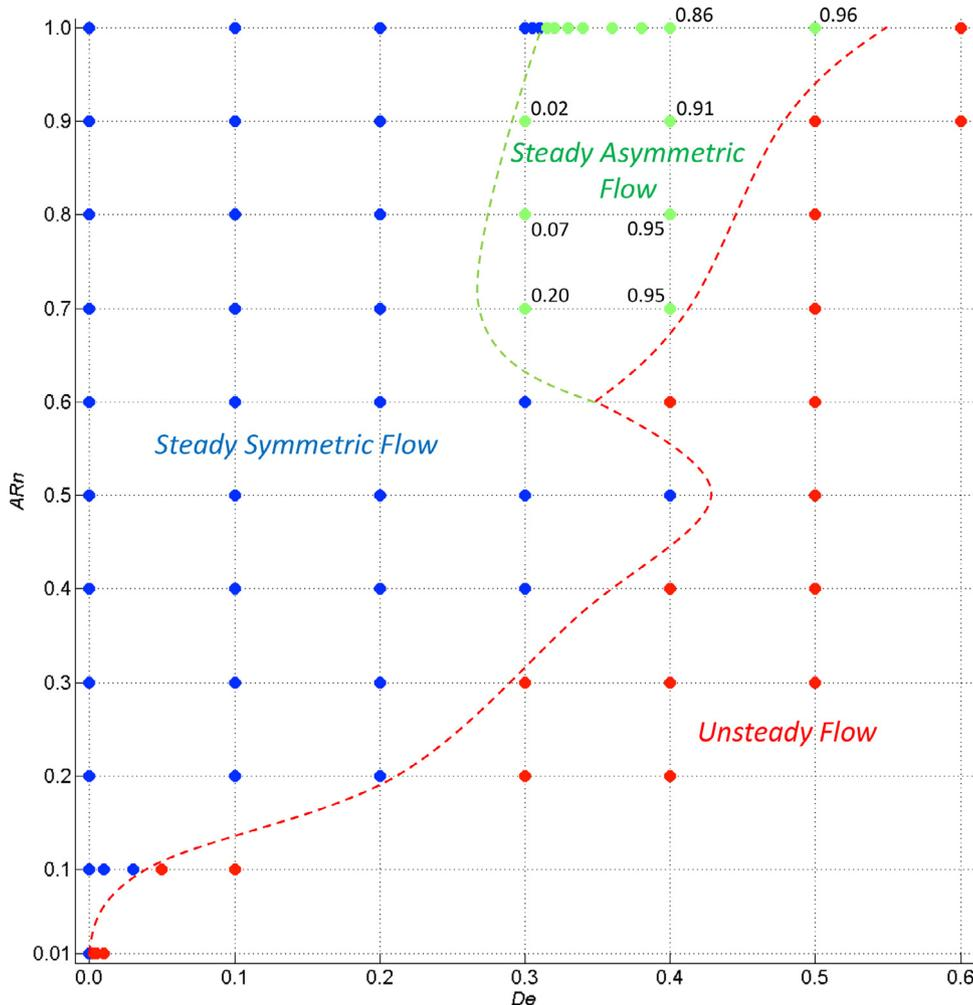
**Fig. 4.** Stability diagram for UCM fluid. Values are given for the cosine of the angle between non-vertical eigenvectors  $(\hat{v}_1, \hat{v}_2)$  of  $\nabla \mathbf{u}^\dagger$  at the centre of the cross-slot. The dashed lines are a guide to the eye.
