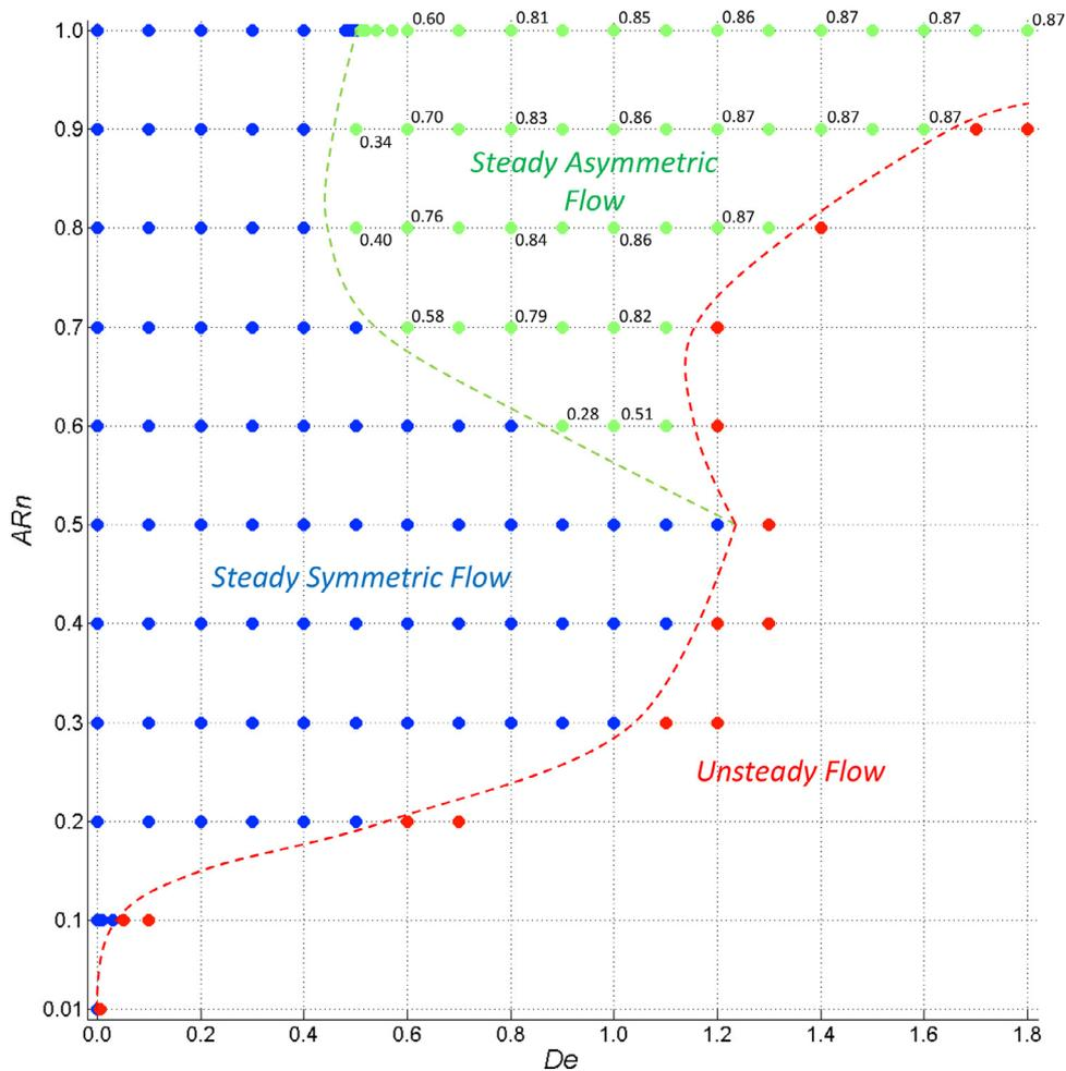
Fig. 5. Stability diagram for sPTT fluid with  $\varepsilon = 0.02$  and  $\beta = 1/9$ . Values are given for the cosine of the angle between non-vertical eigenvectors ( $\hat{\mathbf{v}}_1, \hat{\mathbf{v}}_2$ ) of  $\nabla \mathbf{u}^T$  at the centre of the cross-slot. The dashed lines are a guide to the eye.
