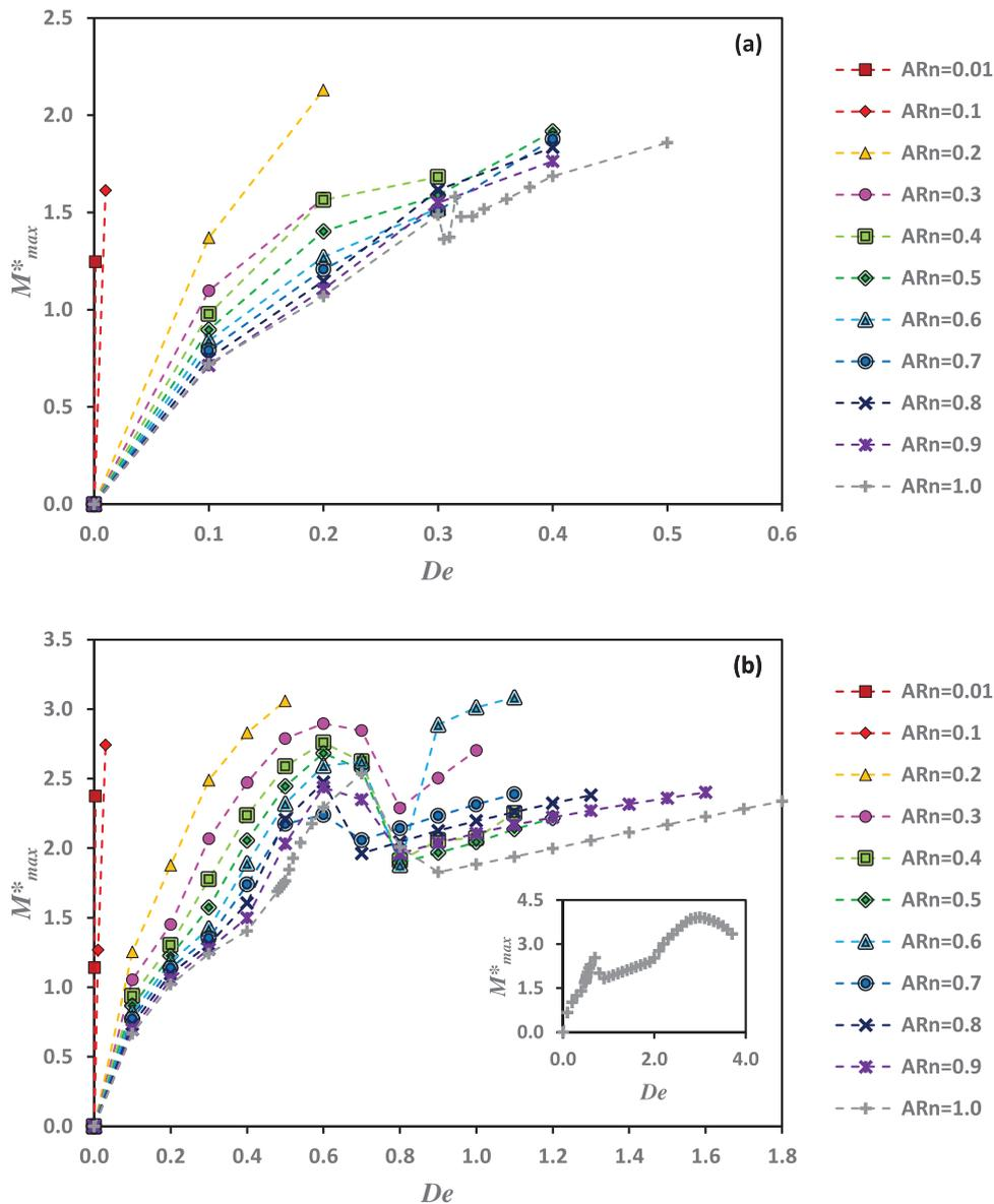
Fig. 11. Maximum value of the modified Pakdel–McKinley criterion  $M^*_{max}$ , for the (a) UCM and (b) sPTT models, the latter with  $\epsilon = 0.02$  and  $\beta = 1/9$ .
