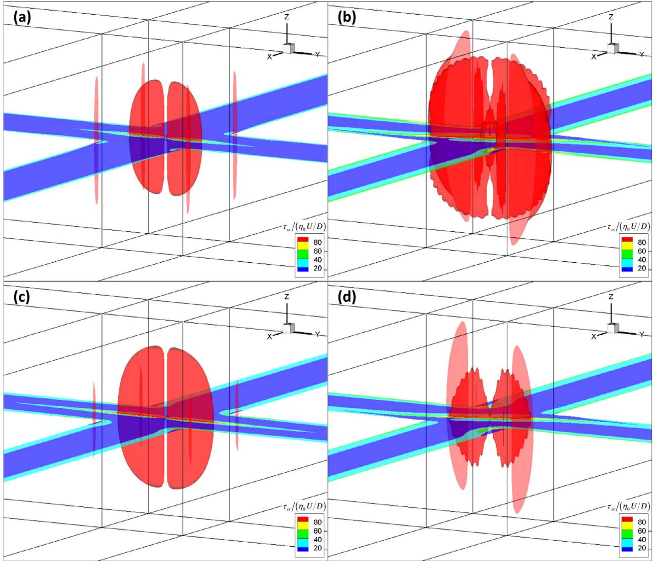
**Fig. 10.** Iso-surfaces and XY centre plane of the normalized streamwise stress  $\tau_{ss}/(\eta_0 U/D)$ , for  $ARn = 0.7$ . (a) Symmetric UCM flow at  $De = 0.2$ . (b) Asymmetric UCM flow at  $De = 0.4$ . (c) Symmetric sPTT flow at  $De = 0.5$ . (d) Asymmetric sPTT flow at  $De = 1.1$ . Iso-surfaces are drawn at  $\tau_{ss}/(\eta_0 U/D) = 80$ . sPTT fluid with  $\varepsilon = 0.02$  and  $\beta = 1/9$ .
