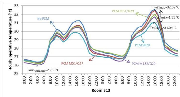
Fig. 6 – Hourly variation of operative temperature on the 22th and 23th for room 313 for the scenario1.
