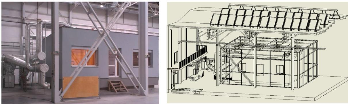
Fig.5 – The 55 m<sup>2</sup>VUKONZE full scale consumer model of house with two rooms.
