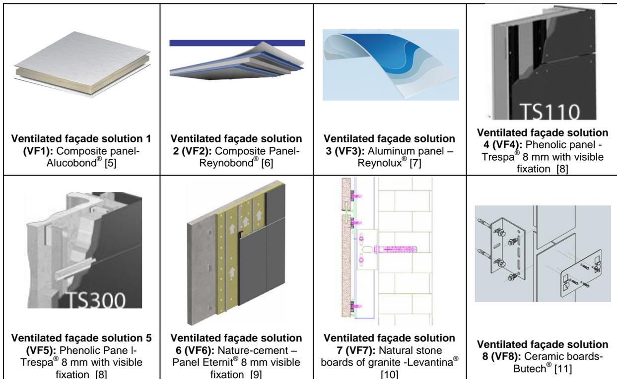
Fig. 2 – The eight solutions of ventilated façades to study in this work.
