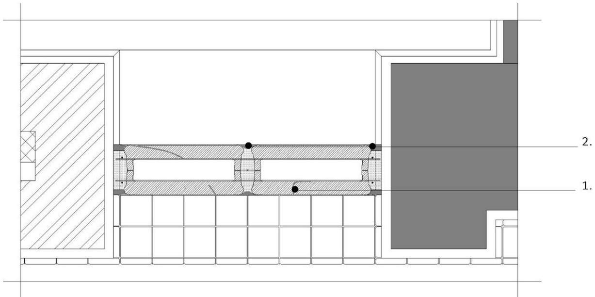
Fig. 3 – Detailed drawing of the constructive reconstitution of the glass brick windows [3].
