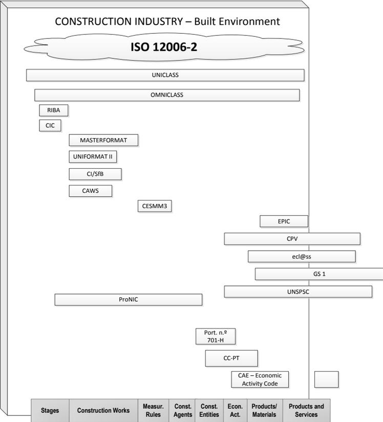
Fig.1 – Schematic overview of the classification systems related with construction [2].
