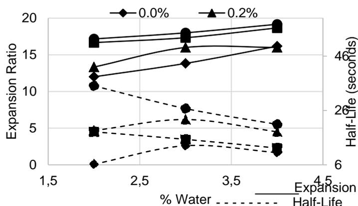
Fig. 1 – Foamed bitumen expansion ratio and half-life results.
