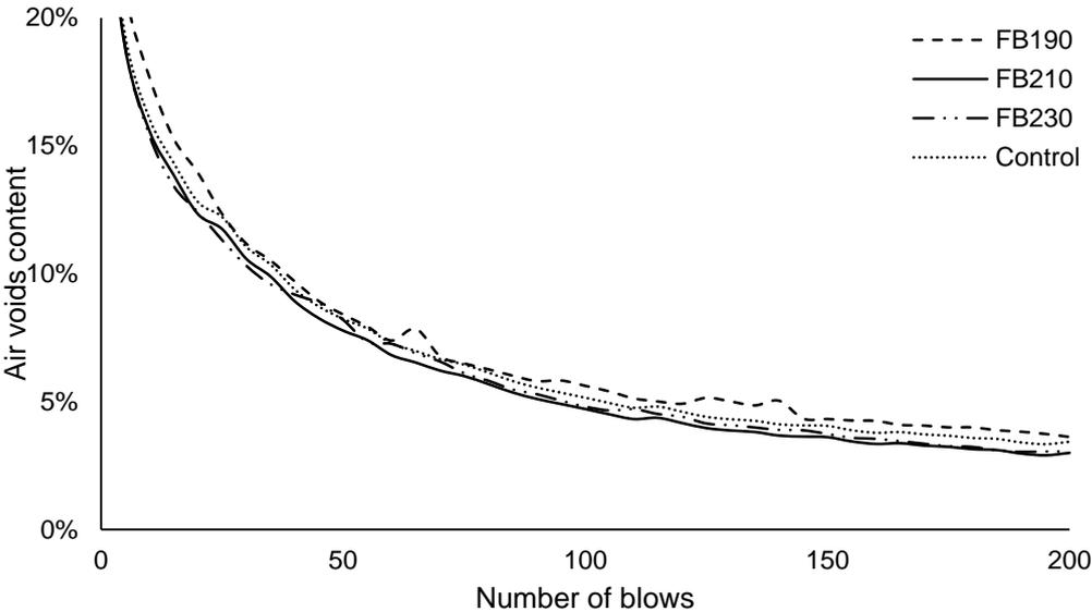
Fig. 2 – Compactability test results of the studied mixtures.
