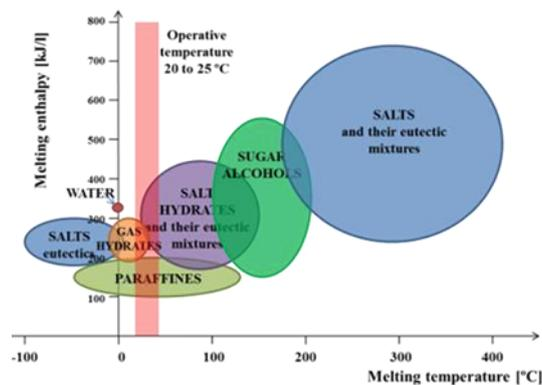
Fig. 1 – Melting temperatures and phase change enthalpy for existing PCMs (adapted from [4]).
