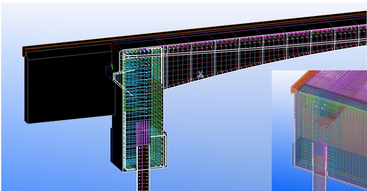
Reinforcement details of the Nahkuri Bridge.
