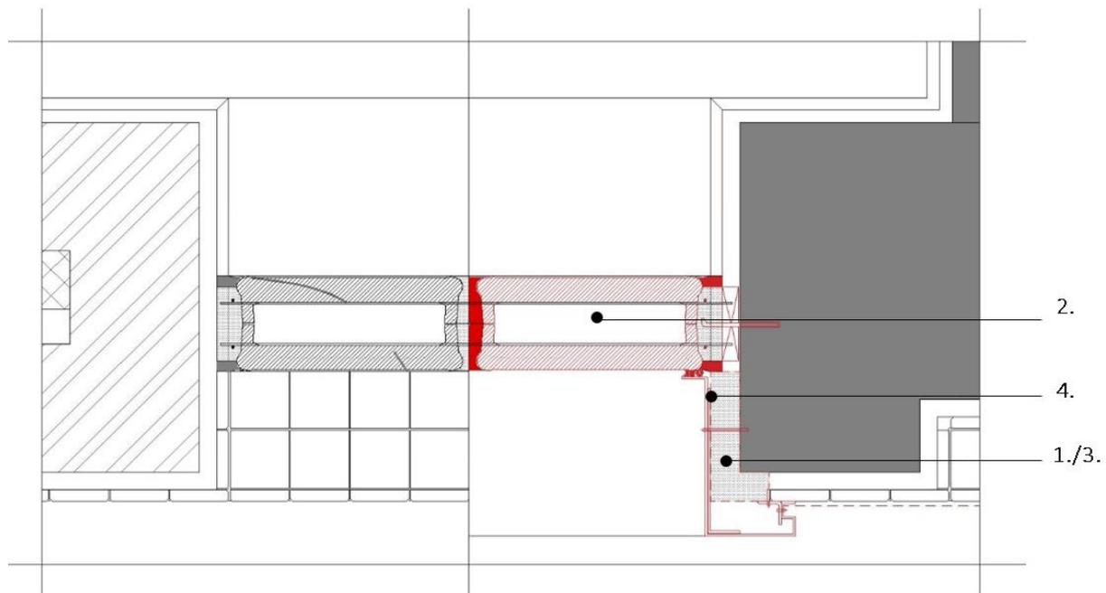
Fig. 6 – Proposed repair approach for glass brick window anomaly [3].
