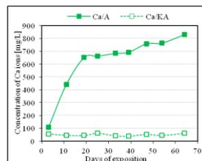
Fig. 8 – Leaching out of Ca ions for samples A (microbial sulphate environment) and KA (a-biotic sample) during 63 days of the experiment.
