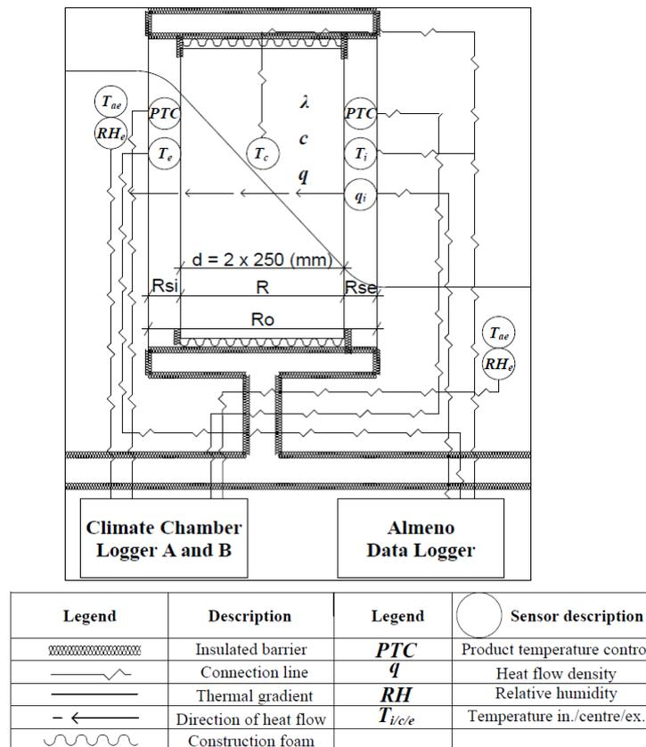
Fig. 9 – Detailed schematic of sensors for the consumer model building envelope & data-logger - Adapted form [1]
