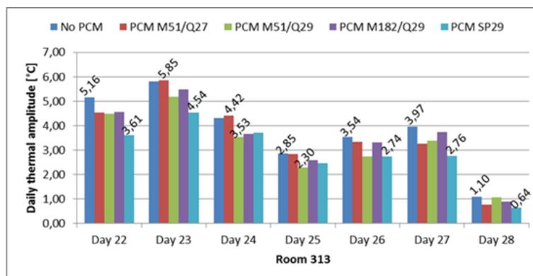
Fig. 7 – Comparison of maximum thermal amplitudes for room 313 with different wall and ceiling coverings, from 22<sup>nd</sup> to 28<sup>th</sup> of July for scenario 1.
