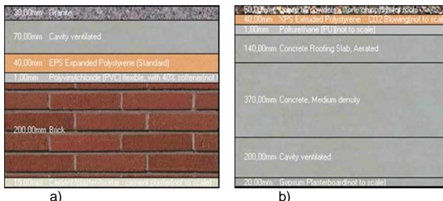
Fig. 5 – Composition of wall façade (a) and ceiling (b) of computer rooms.
