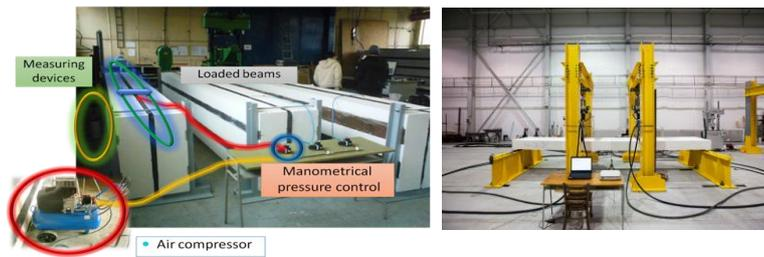
Fig. 4 – Analysis of the resistance of deck bridges with encased steel beams.
