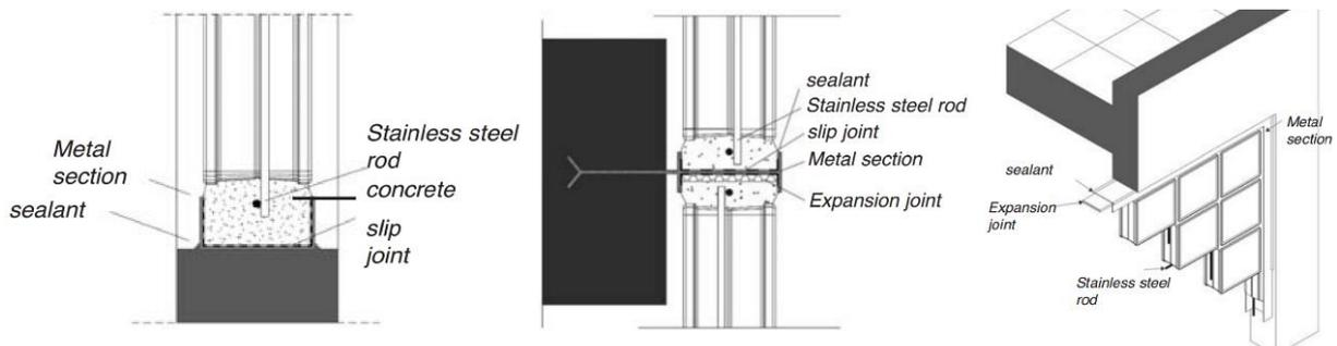
Fig. 5 – Restraining detail examples for glass brick installation with the traditional system (cement mortar) [4].
