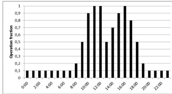
Fig. 2 – Template of operation schedule for computer rooms.
