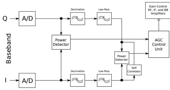
Fig. 4. Automatic gain control logic blocks [23].
