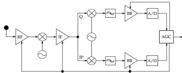
Fig. 3. Typical analog reception chain in 802.11 devices [23].
