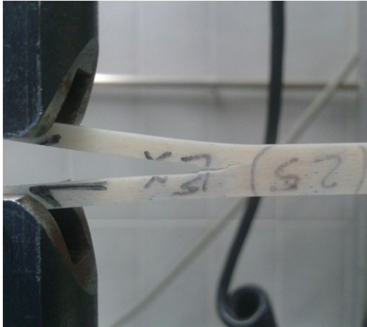
Figure 10. Crack deviation at initiation in a DCB test of human bone.
