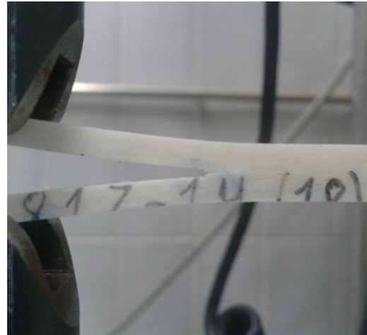
Figure 11. Self-similar crack propagation without deviation from its initial plane.
