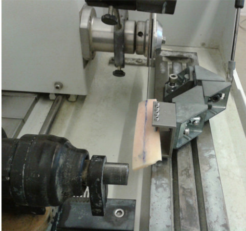
Figure 2. Cutting operations performed to get the final specimens.
