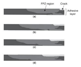
**Figure 5.10** Evolution of damage (crack and FPZ region) inside the adhesive layer in the DCB test. Figures a-d present four steps of the evolution of the crack and the FPZ region inside the adhesive.
