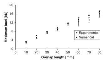
**Figure 5.12** Comparison between numerical (continuum damage model) and experimental single-lap joint strengths in terms of maximum loads as a function of overlap length.
