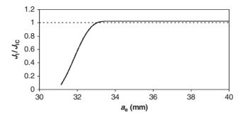
**Figure 5.9** *R*-curve of the DCB test. The horizontal line  $(J_1/J_{1c}=1)$  identifies the value inputted in the model.
