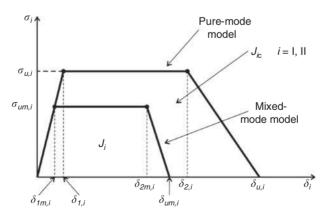
**Figure 5.1** Pure and mixed-mode I+II cohesive damage model.
