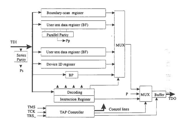
Figure 0-1. Alternative Parity generation circuits
