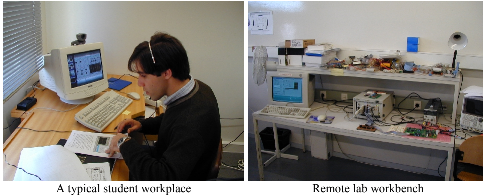
Fig. 3. A student workplace and the remote lab workbench during the interim trials of the digital and mixed-signal test experiments. Notice the PXI server and instruments, all contained in the rack at the center of the workbench
