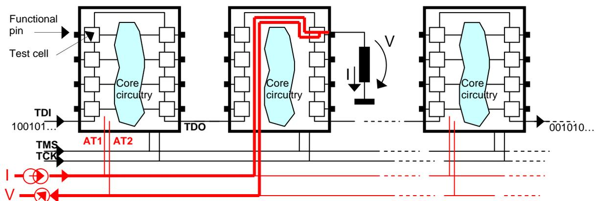
**Figure 1:** Test cells (DBMs / ABMs) and boundary-scan register in an 1149.4 chip.
