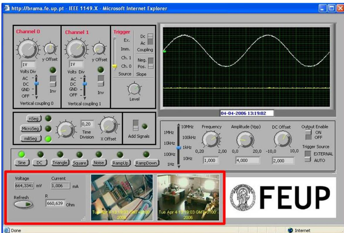
**Figure 9:** Experiment interface window #2 for parametric testing: Oscilloscope, waveform generator, multimeter, live images from the remote lab. Notice that the oscilloscope and the waveform generator are not used in this experiment.
