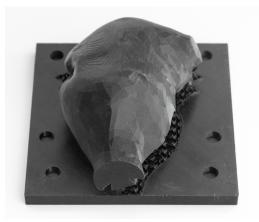
Figure 3.7: Photograph of the final 3D-printed PLA mold, printed in two halves. The remaining portion of the front part is shown on the left, and the back part on the right.
