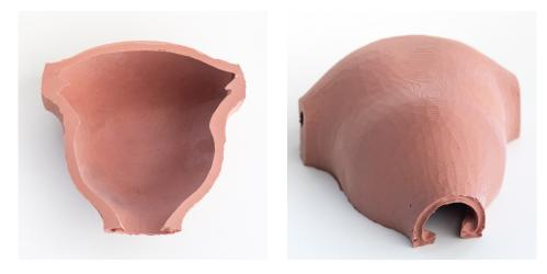
Figure 3.8: Final silicone uterus model captured after demolding. The anterior view is shown on the left, and the posterior view on the right.
